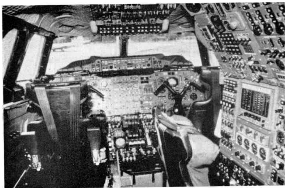
Fig. 2. (a) Flight deck display on Concorde 002—the first British prototype. This is a striking example of the use of electronics to absorb a mass of information, analyse and present it.
