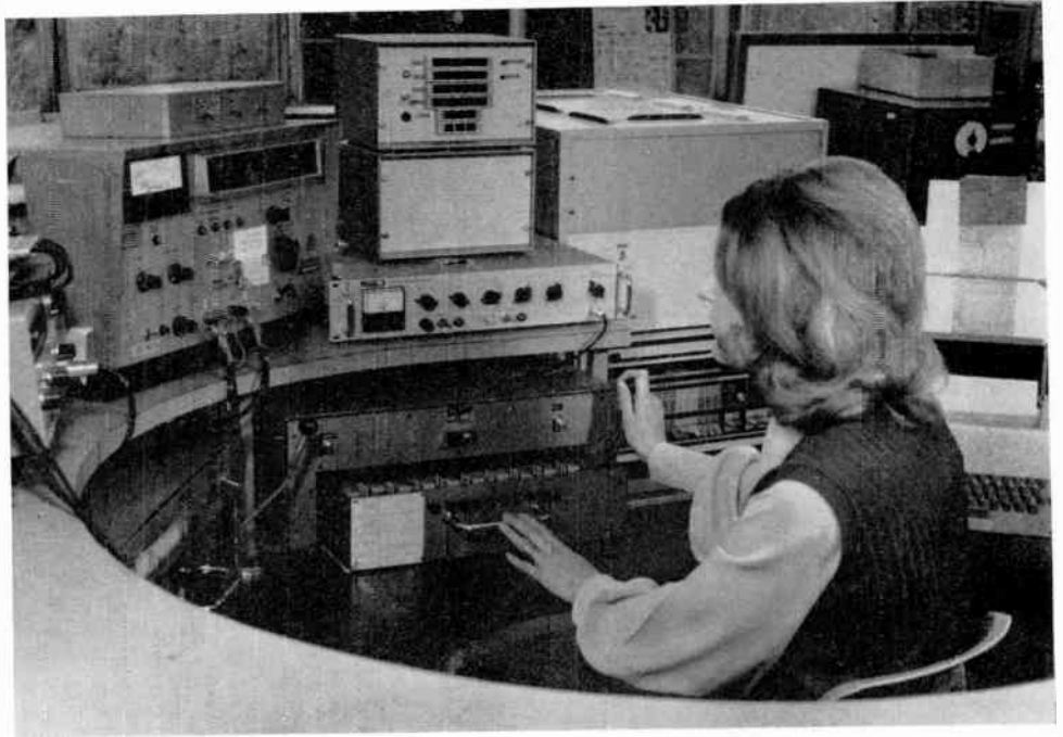
Fig. 7. Automatic test equipment with computer control.
