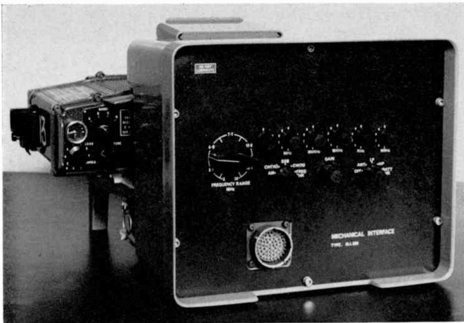
Fig. 2. One of the electro-mechanical interfaces to be used as part of the Clansman field test console.
