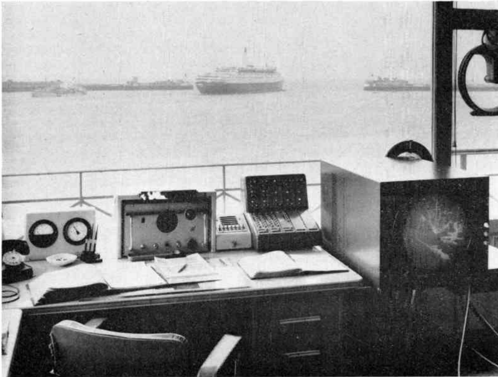
(a) Operations room at Le Havre, showing experimental scan-conversion display.
