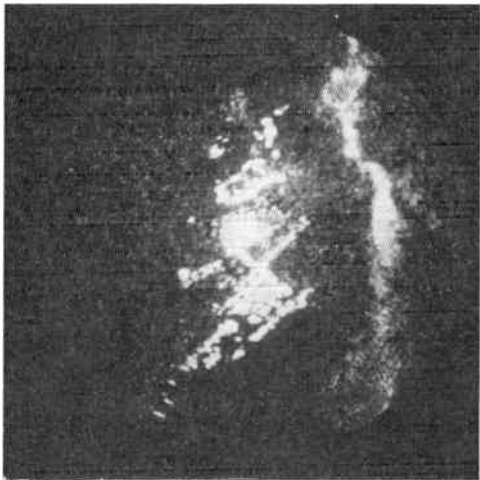
(d) As Fig. 8(c) but with side-lobe suppression in operation. Rain clutter band extending.
