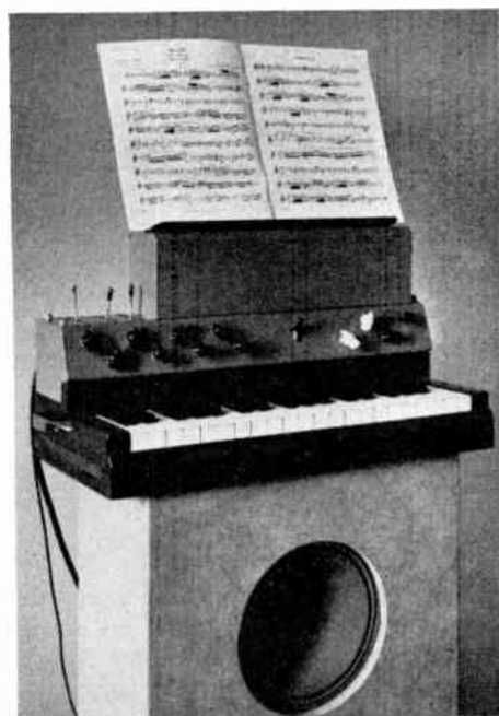
Fig. 3. Electronic melodic instrument demonstrated at the lecture. The three controls for the left hand are for loudness, depth of vibrato and 'muting', respectively. The panel controls affect formants, harmonic series (natural or even numbers), attack, vibrato speed, pitch range, etc.
