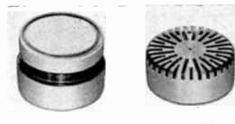
Fig. 1. A condenser microphone cartridge (left) with its protection grid removed (right).
