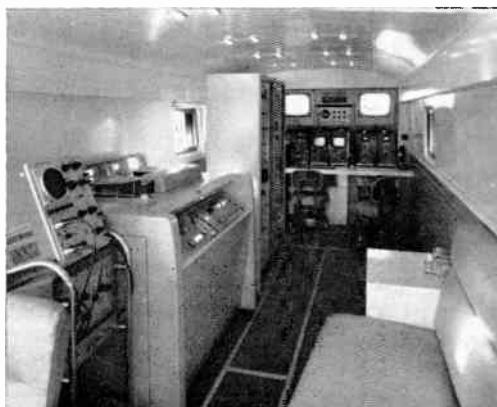
Fig. 2. The inside of the vehicle. The Videotape recorder is at the left foreground and the camera control and monitoring equipment in the background.
