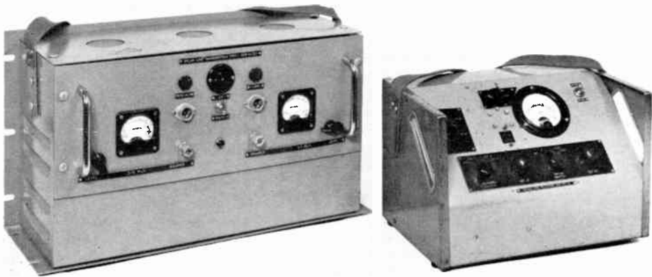
Fig. 8. Network transmission measuring equipment. Mains-operated twin transmitter (left) and Portable receiver (right).
