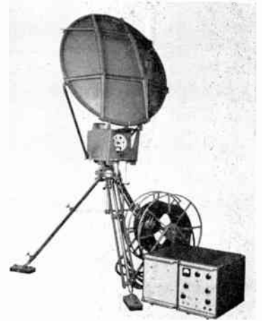
Fig. 8. (above) Transmitter receiver; aerial, head, transmitter or receiver unit, and power supply unit.
