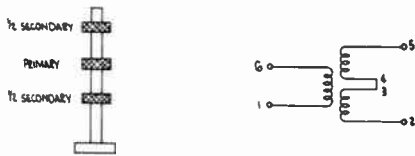
Fig. 7. Details of "pulse" transformers. Standard Aladdin former. Wire—40 SWG EN SS covered. Coil width 3/16". Douglas Wave Winder Gears: A, 48; B, 32; C, 34; D, 50; E, 40; F, 80.
