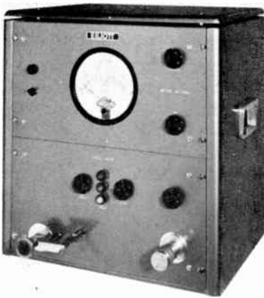
Fig. 5. The automatic standing-wave indicator.
