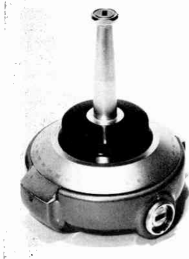
Fig. 1. The rotary standing-wave indicator.
