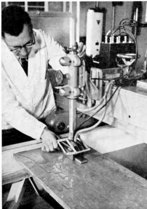
Fig. 19. Gap scanning of plate material.
