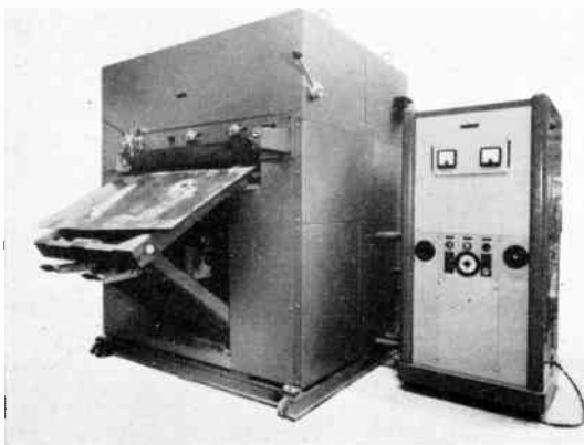
Fig. 16. Machine and associated r.f. generator with loading carriage down and petrol tank sheet and fittings in position. (Courtesy Vauxhall Motors Ltd.)
