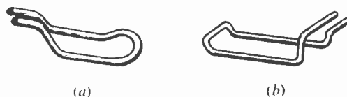
Fig. 3. (a) Hairpin coil. (b) Skid coil.
