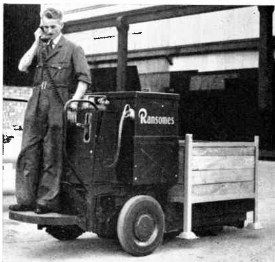
Fig. 1.—Transmitter-receiver installed on an electric truck.
