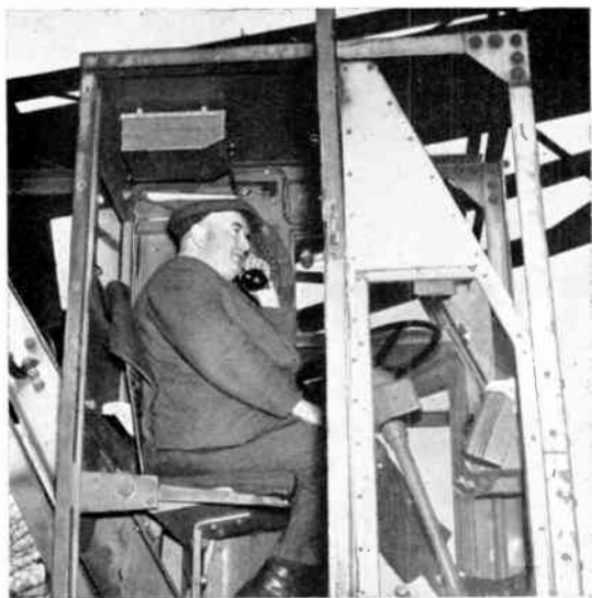
Fig. 2.—Transmitter-receiver installed in roof of cab of a 6-ton mobile crane.
