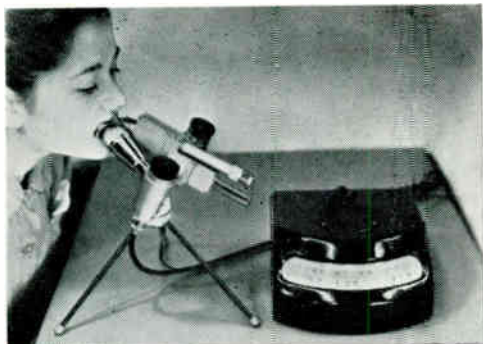
Fig. 5.—Reflectometer-type transducer used in dentistry to compare whiteness of teeth.
