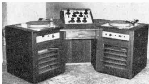
Fig. 21.—Typical studio control desk showing mixer panel.
