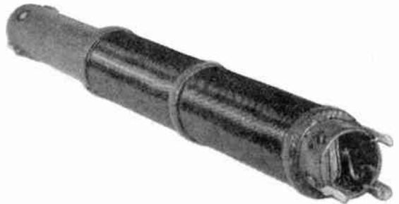
Fig. 15.—Typical vacuum cleaner suppressor.
