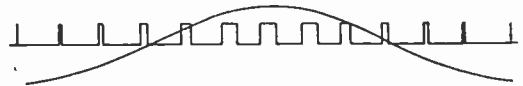
Fig. 15.—Signal and corresponding "variable width modulation." The variable width modulation is usually derived from the time modulation at the receiver.
