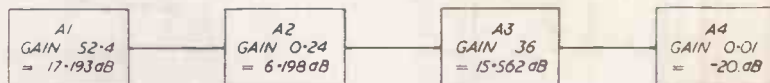
Fig. 1. Block diagram of amplifier and attenuator chain. Input/output ratio = 52.4 \times 0.24 \times 36 \times 0.01 = 4.53 . In decibels, input/output ratio = 17.193 - 6.198 + 15.562 - 20 = 7.294 \text{ db} = 4.53 .
