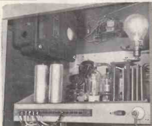
The output from the 50-watt DET18 triode valve under test, centre, illuminates the tungsten lamp, right. When the output, at the end of the test, falls off the lamp fades and causes the photoelectric device, left, to operate a timing device which records the number of hours run.
