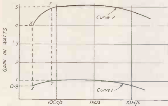
Fig. 3. (Left) Response curves on linear gain scale. The percentage drop at "X" compared to "Y" is the same in both cases, though not directly apparent. (Right) The same response curves on a decibel scale gives better comparison of levels.
