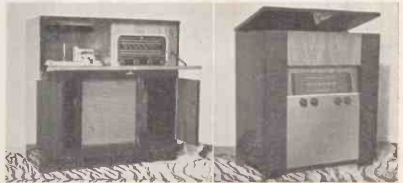
Two new Ronden radiogram models: left—Model DRG948 bureaugram, and right—Model 533ARG console radiogram. The bureaugram incorporates a v.h.f.-f.m. band.
