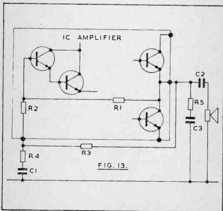
In Fig.13 the output stage provides negative feedback via R1 to a stage in the input part of the IC. R1, together with R2, and the external components R4 and C1, largely determine the feedback used. R3 may be added as an external component, or may not be present.
