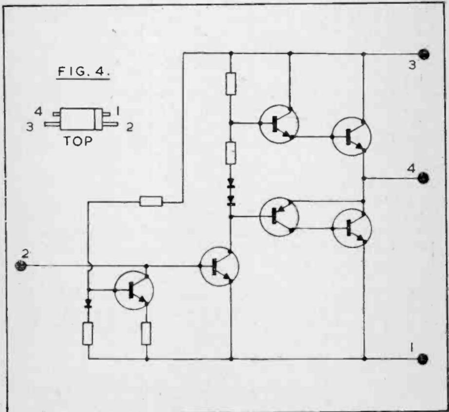
The equivalent circuit, Fig.4, contains one PNP and five NPN transistors, with three diodes and five resistive elements. Basically the device is a driver stage followed by push-pull output, with stabilisation of working conditions. Audio input is between points 2 and 1, with output between points 4 and 1. Point 1 is also the negative line, and point 3 the positive line.
