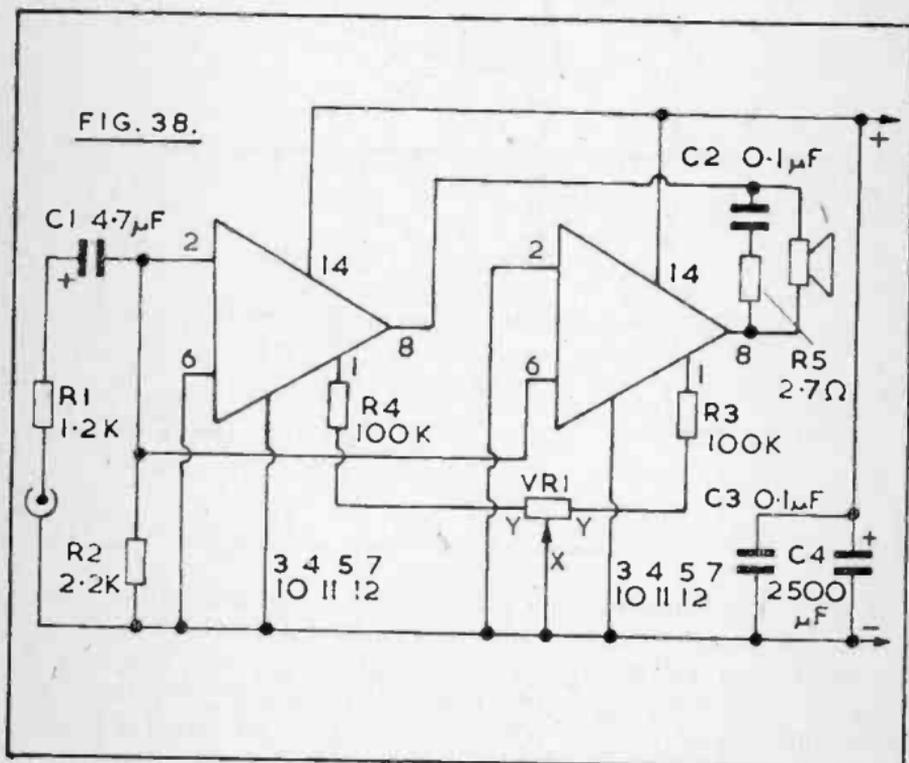
C3 across C4 is to help avoid HF instability (possibly not audible) which will cause heavy current, but very poor reproduction. The speaker and output circuits should be removed from input circuits, for the same reason.
