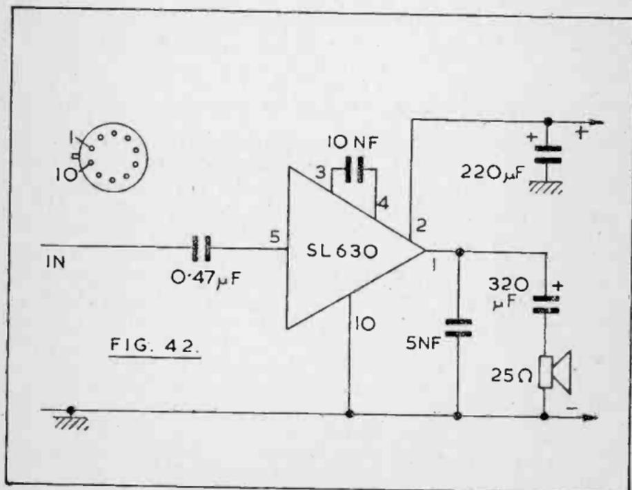
This small audio IC can be used with up to 12v, giving adequate power output for headphones, or speaker reproduction for relatively low volume purposes. Fig.42 is a simple circuit. Current drain is about 10mA, with about 150mW output.
