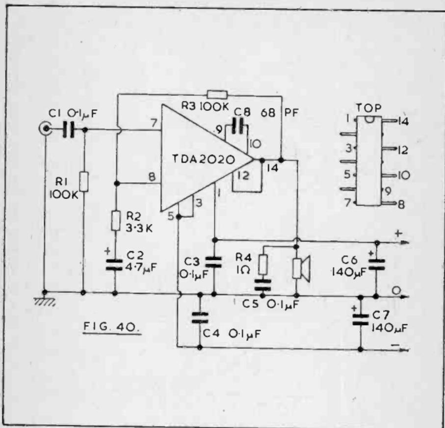
A split power supply is required, but can be readily arranged as shown later (Fig.51). Minimum output rating of this IC is 15w with a supply providing 17-0-17v and 4 ohm speaker, the typical rating being 18.5w. With an 18-0-18v supply, typical outputs are 16.5w for an 8 ohm speaker, and 20w for a 4 ohm speaker. Sensitivity for 15w output is 260 to 380mV input. Input impedance is 1 megohm.
