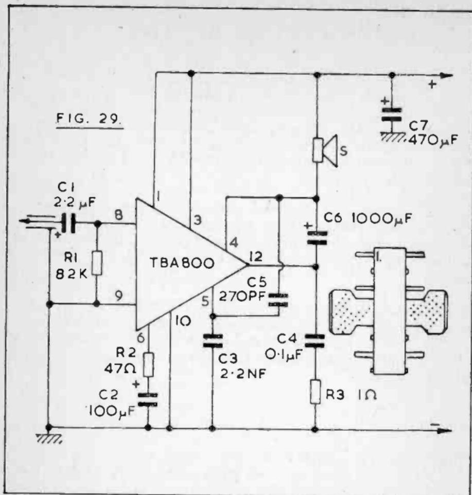
For outputs of over 1W, the tabs must be soldered to a heat sink. This can be arranged by passing them down through slots in a printed circuit board, so that they can be soldered to an area of at least 2 x 2 in (50 x 50 mm) provided on the board. Tags fit 0.1 in matrix board; or 0.15 in matrix if the IC is placed diagonally.
