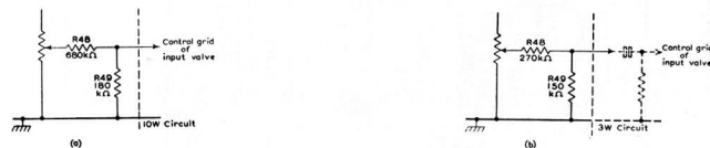
Fig. 1—Output-attenuating networks for use with both pre-amplifiers
