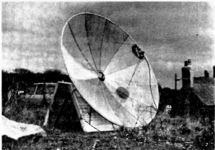
A home constructed 5 foot diameter parabolic dish used for satellite reception experiments
