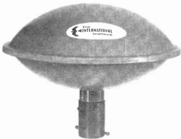
A wideband VHF/UHF 'active aerial', intended for marine use. Some 20" in diameter, it features an integral wideband amplifier of some 27 dB gain, noise 5.5 dB and coverage of 40-860 MHz (Aeramics Electronics Ltd, Peterhead)
