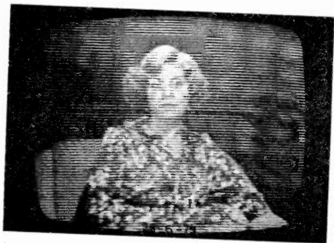
An example of Band 3 Sporadic E propagation. The announcer is from RTA Algeria on ch. E5 and received in the Netherlands. Note the additional 'floating' signal in the background on the 5544 test card
