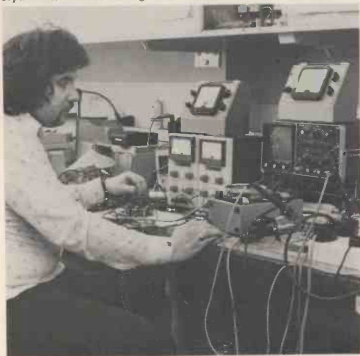
Equipment is tested and repaired in the maintenance room.
