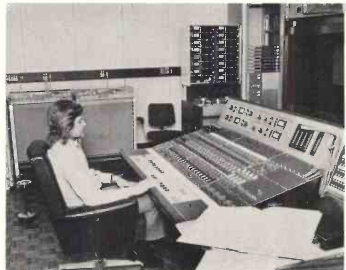
A mixing room with Mike Fitz-Henry at the Neve console desk. Note the Studer tape machines and the Dolby noise-reduction units on the far wall.
