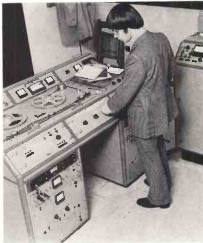
The cutting room featuring the amplifier, Dolby unit and the ASRA phase-correction unit. The lathe is an Ortufon. Alan Corbeth, formerly of Bell Records, at the controls.
