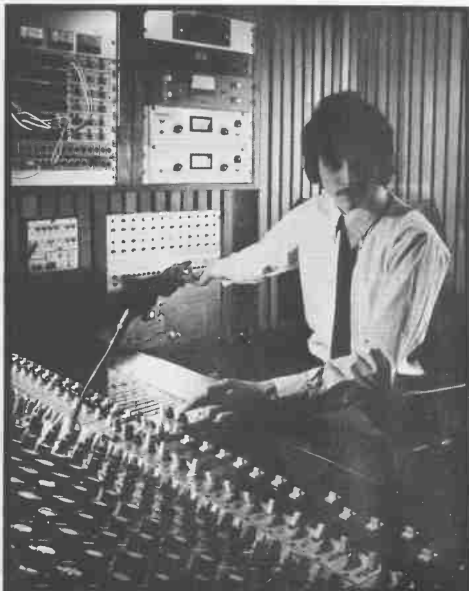
Robin Cable at one of the Sound Techniques' mixing desks used at Trident Studios, now equipped with twenty-two A301 units on two sixteen track machines.
