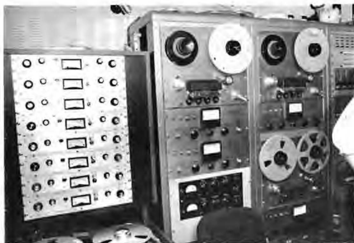
Lansdowne 8 track machine on the left with playback panel on the right.
