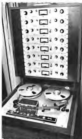
Note the wide tape necessary for 8 track recording.
