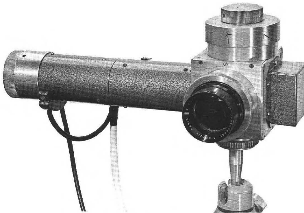
Fig. 10 — Photograph of photoelectric tristimulus colorimeter head
