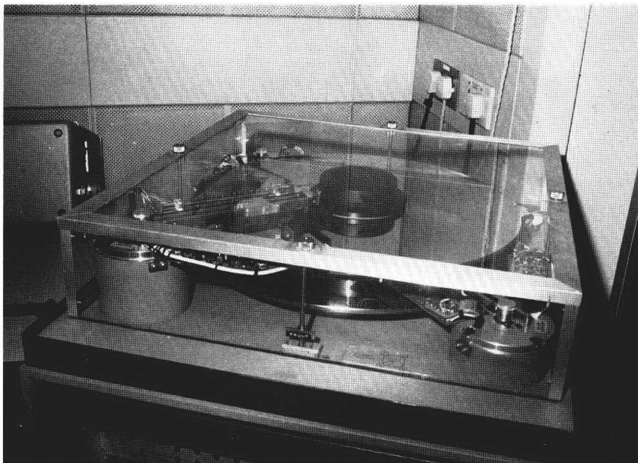
Fig. 1 Video disk motor unit showing tracking mechanisms
