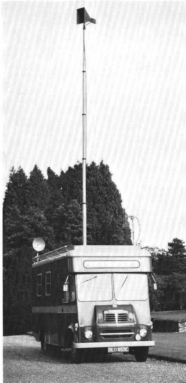
Fig. 3 The measuring vehicle, showing the telescopic mast fully extended with the horn aerial in position
