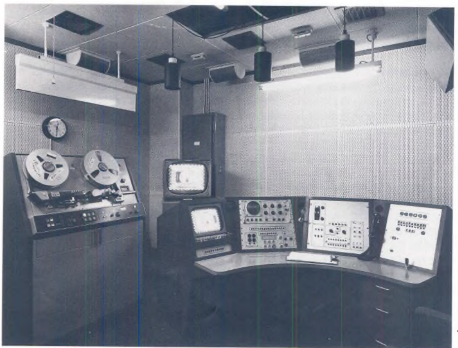
1966: An Ampex VR2000 quadruplex videotape channel at TC
