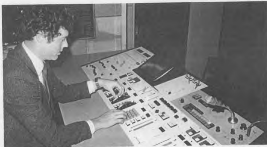
The lighting desk in studio 8 undergoing tests by Mike Wolfe of SCPD
