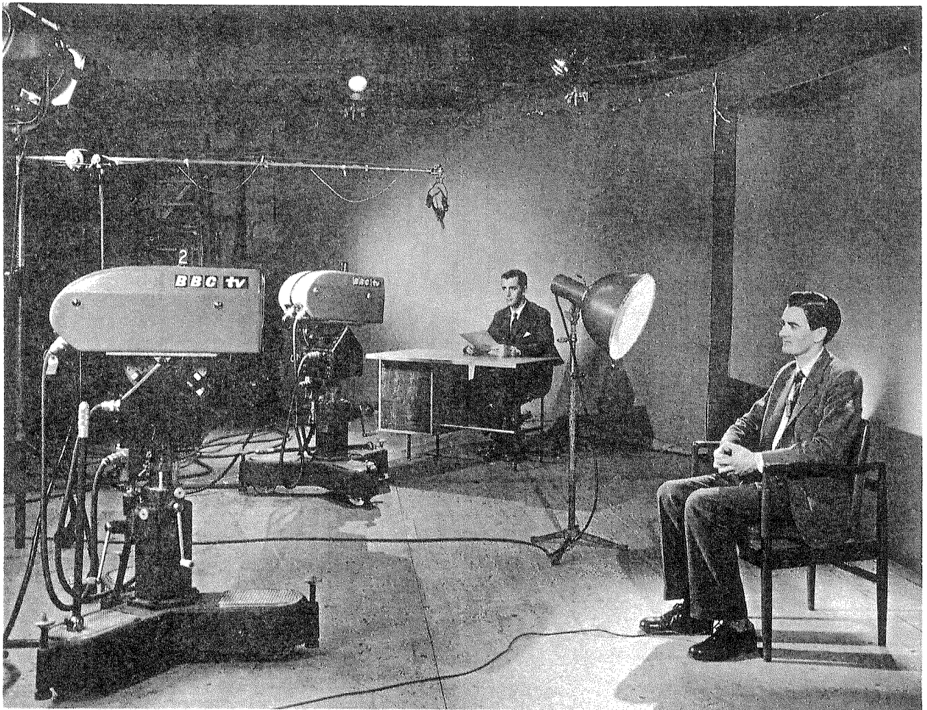
Plate 13 — Remotely controlled vidicon cameras in the News Studios at Alexandra Palace
