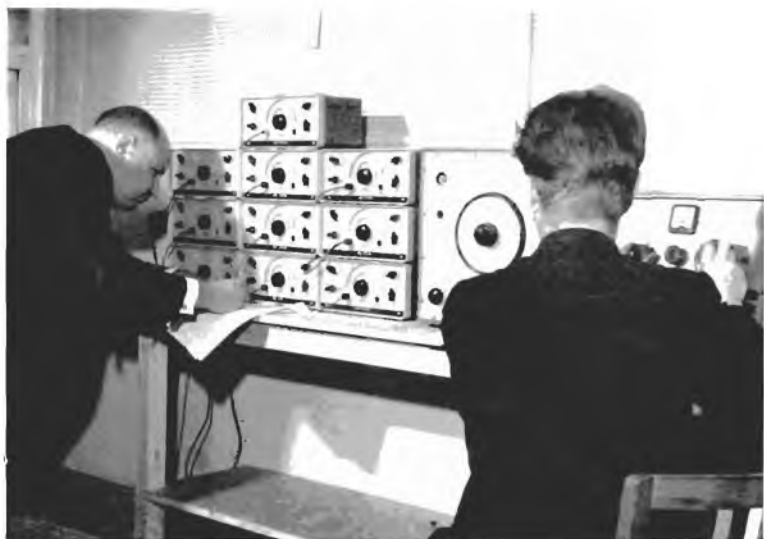
Plate 15.5. Bank of oscillators, showing use of frequency standard (on right) to set up accurate combinations of tones
