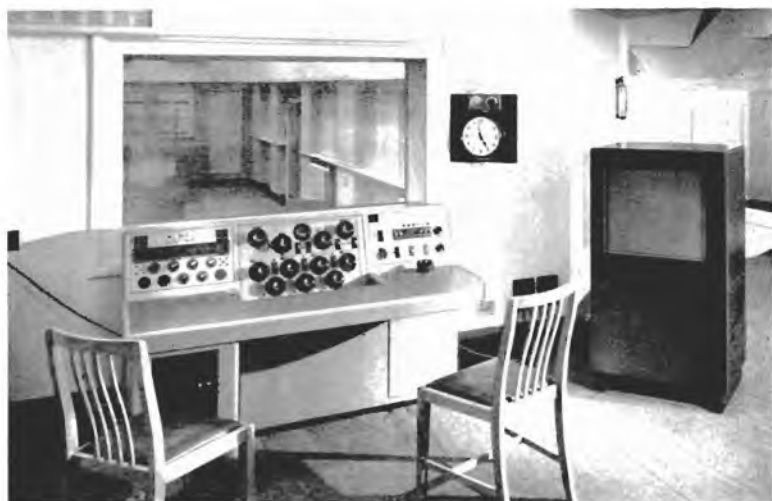
Plate 6.1. Studio control cubicle showing loudspeaker unit LSU|10
