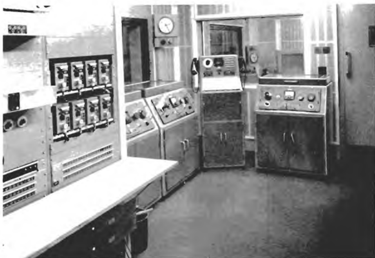
Plate 10.6. Engineer's control cubicle at the Paris studio in London, showing, in addition to the normal control bay, the three tape recorders for local recording. The Studio Manager's control cubicle can be seen through the far window
