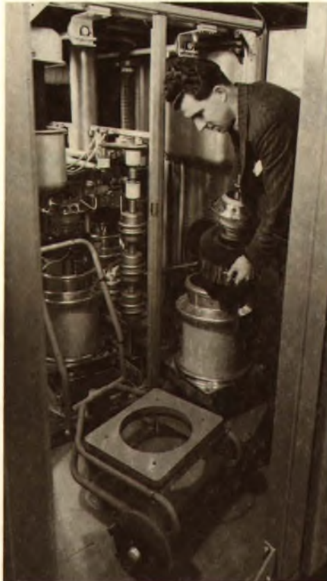
Left: Changing a valve on the Third Programme transmitter, 1950.
