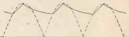
Fig. 6.—Full-wave output for 4-microfarad reservoir capacitor
