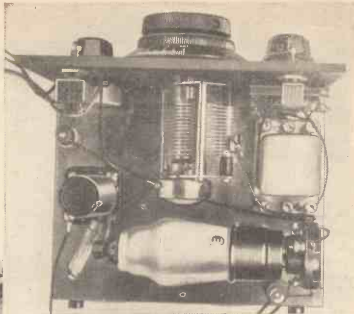
As this plan view shows, the high-frequency pentode valve is fitted horizontally to save baseboard space. Just by the valve holder is the high-frequency bypass condenser
