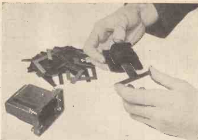
Although this is not a mains transformer but only a low-frequency-coupling model, the fundamental construction is the same—with laminations inside the wire bobbins
