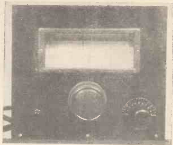
As you can see from this front view of the control panel, there are very few knobs to twiddle. A wide-vision scale helps to log stations accurately
