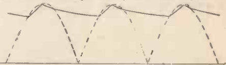
Fig. 5.—Output from full-wave rectifier
