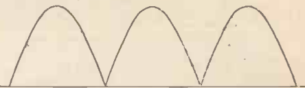
Fig. 5.—Output from full-wave rectifier
