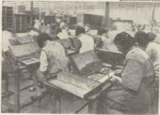
Here you see the girls soldering small sockets on to the zinc containers for the high-tension and grid-bias batteries
