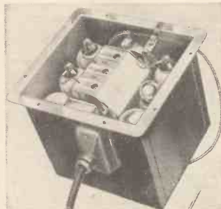
Neat and compact, isn't it? A good view of the Lissen car-radio six-valver, showing the extension cable at the front
