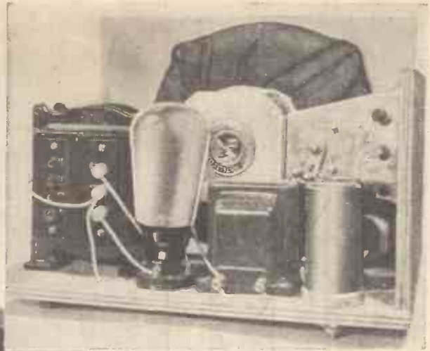
Another view of the A.C. Penta-quester mains unit with the rectifying valve fitted in position near the transformer
