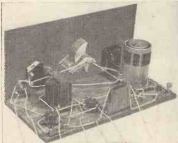
As you can see from this picture, the tuning coil is mounted at the extreme end of the baseboard, with the three valve holders in line along the back.
