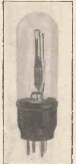
A mercury-vapour lamp of the type shown by the diagram
