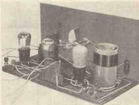
There is plenty of room to spare, even when the three valves have been fixed in their holders, as in this view of the back of the completed set. Note the two terminal blocks
