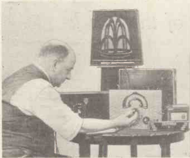
Testing the "A.W." Short-wave World-beater in Cornwall—checking the stations by means of a wavemeter
