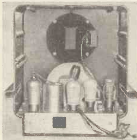
When you take the back off the Ekco B54 you see a clean metal chassis, with moving-coil loud-speaker chassis above
