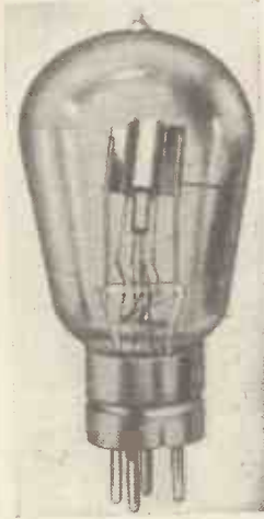
The old type KLI—the first indirectly-heated cathode mains valve
