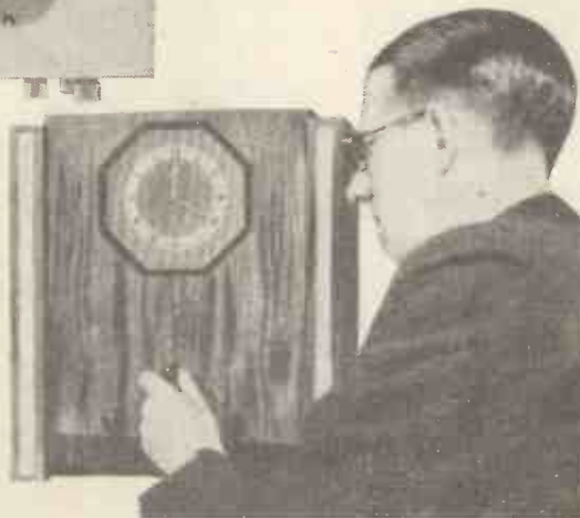
Our man tuned-in a station on the gang condenser knob—but note the clock-face dial providing a new! alternative method of station logging
