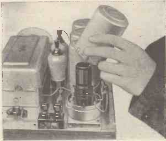
Many of the components in a modern receiver are provided with their own screens. Note that there is good clearance between the coil and its can
