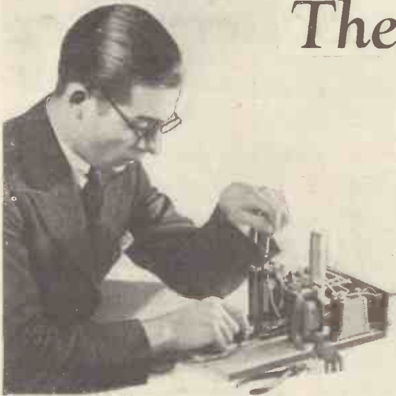
Completing the assembly of the D.C. mains unit described in this article. Two home-made smoothing chokes are used—and they can be made very cheaply
