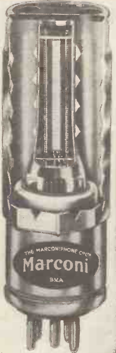
How the electrodes are rigidly arranged in a Catkin valve
