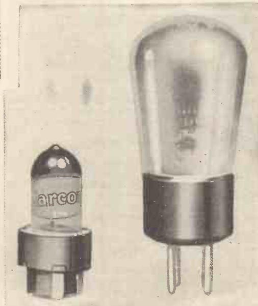
One of the new Marconi 1-volt midget battery valves photographed by the side of a standard type
