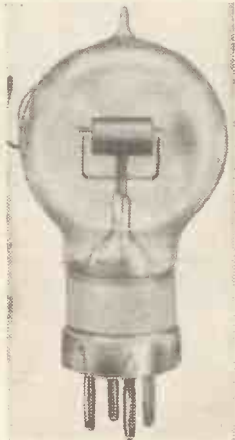
One of the original R (bright-emitter) valves
