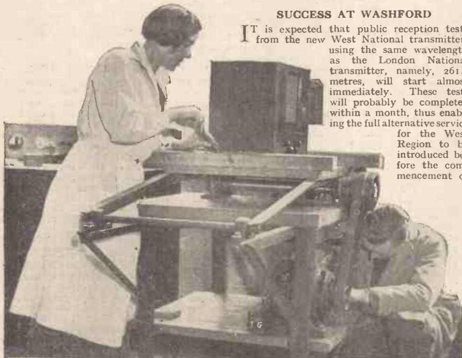
This artificial "train" has just been set in operation at the Research Laboratory of H.M.V. It is used for testing radio sets by vibrating them and a set can undergo vibrations similar to a rail journey from London to Glasgow in twenty-six minutes—932 m.p.h.!
