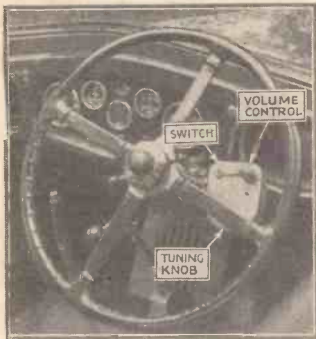
Special control box for operating the set's knobs from the car's steering column. Below can be seen a suggested position for the loud-speaker and on the facia board are the low-tension points from the car accumulator
