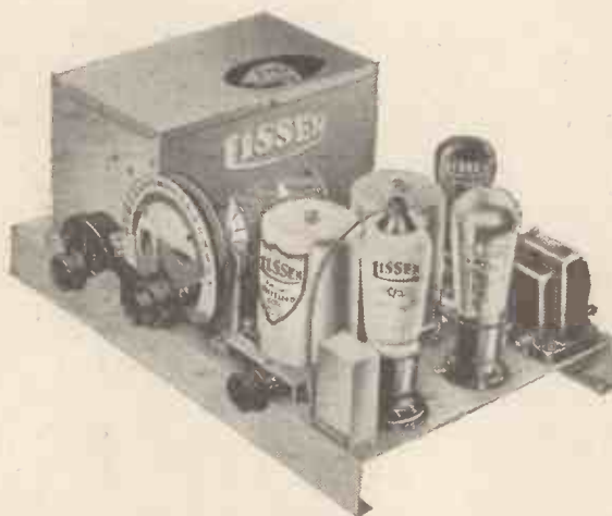
Metal chassis of Lissen A.C. Skyscraper with safety power unit on the left
