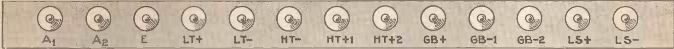
A composite terminal strip drawn to show all the terminals usually found on battery sets
