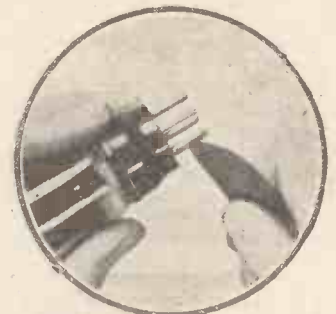
Carefully open out the split pins of valve bases to ensure a good contact with the valve-holder sockets. Take care not to damage the connecting wires that run through the pins
