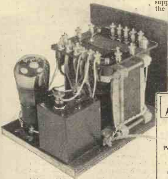
The rectifier and transformer unit which will allow of the D.C. unit being used on A.C. mains
