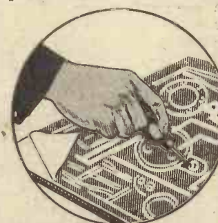
Prick through the screw holes in the full-size blueprint when fixing the baseboard components
