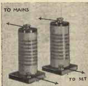
Two high-frequency chokes can be connected, one in each mains lead, in order to cut out interference induced by the mains
