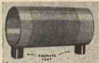
Here is a good coil-mounting hint. Small feet are cut from lengths of ebonite to stand the coil away from the baseboard
