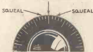
The best test to determine whether you are tuned to the silent point of oscillation is to turn the dial each side of the tuning point. If there is a squeal you must reduce reaction
