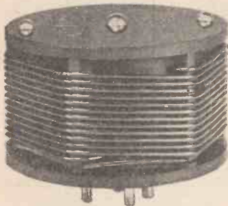
One of the short-wave coils used in the Aerodyne Adaptor
