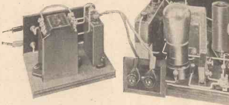
The unit connected to the set speaker terminals
