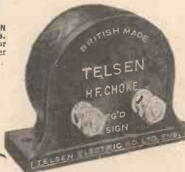
TELSEN H.F. CHOKE. Specially selected for the 1931 Ether Searcher. Designed to cover the whole wave-band range from 18 to 4,000 metres. Extremely low self-capacity, shrouded in genuine Bakelite. Inductance 150,000 microhenries. Resistance 400 ohms. Price 2/6 each.
