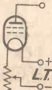
Fig. 4. Use is made of a rheostat in the filament lead of the screen-grid valve in this arrangement
