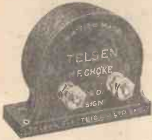
TELSEN H.F. CHOKES. Designed to cover the whole wave-band range from 18 to 4,000 metres, extremely low self-capacity, shrouded in genuine Bakelite. Inductance 150,000 micro-henries. Resistance 400 ohms. Price 2/8 each.
