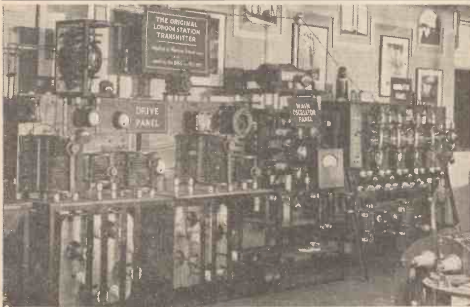
Compare this with the Brookman's Park gear! Listeners who went to the Show saw this original 2LO transmitter in the B.B.C. exhibit. It is the transmitter used by the B.B.C. from 1922 to 1925, and has a power of 1\frac{1}{2} kilowatts
