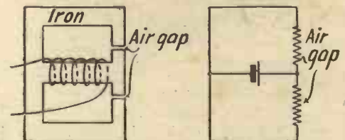
Fig. 2.—Magnetic circuit and equivalent electrical circuit
