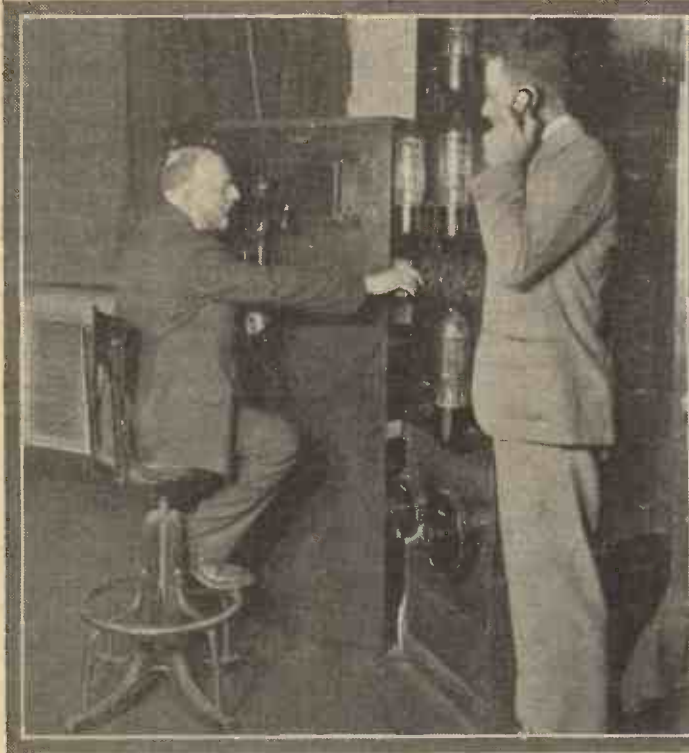
The sitter is almost surrounded by the large sheets of diffusing glass, behind which are the colour-sensitive photo-electric cells. Dr. H. E. Ives is seen seated in the left-hand picture
