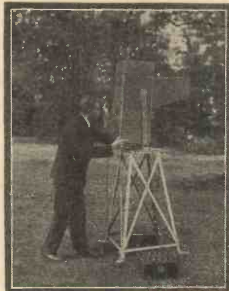
A view of the Noctovisor invented by Mr. J. L. Baird. There is a small circular screen on which the lights are made visible. A graduated scale at the base of the instrument gives their exact bearing in relation to the Noctovisor.
