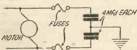
Fig. 3. A D.C. Smoothing Circuit
